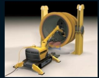
Continue by enlarging the V-shape until the base is approximately one meter wide. This decreases tension between the bricks, making the bricks easier to remove. Tearing too much out may cause the bricks to fall in an uncontrolled fashion, which will require the unnecessary emptying of the ladle.
