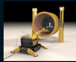
We break out the refractory from the bottom of the ladle. Starting from the lowest part, we work upwards, row by row. When about 60 percent of the refractory has been torn down the rest falls down. Empty the ladle.
