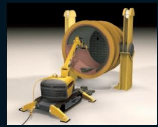
We then tear down the remaining bricks. Thanks to the precise remote-control and the adjustable hammer impact, the working lining can be demolished without causing any harm to the safety lining. Remove the demolition material from the ladle.
