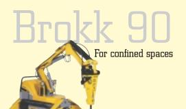
The Brokk 90 is one of the the most versatile demolition tools on the market. It folds into a compact package, can be brought to the site in a small lorry or on an ordinary trailer, go into the elevator or climb stairs, be plugged in and ready to work in an instant. Front and rear flap down outriggers provide exceptional stability. The Brokk 90 is the obvious choice for indoor demolition where there are load restrictions on floors,but where a powerful, labour-saving tool is needed.
